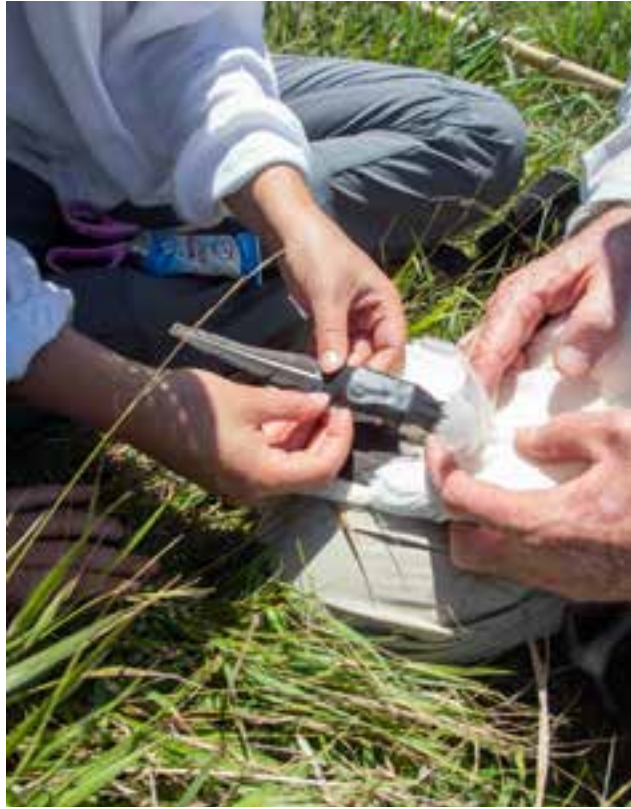
Figure 70. Tail-mounted GPS logger attached to central tail feathers of an Australasian Gannet. Photo: Edin Whitehead.
