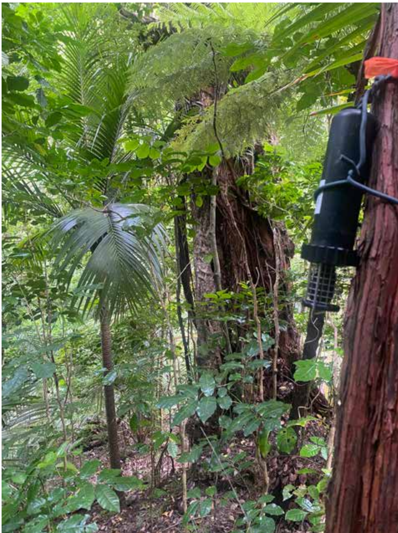
Figure 35. One of the DOC acoustic sensors attached to a tree. The cage over the microphone protects it from being damaged (e.g. by parrots). Photo: Chris Gaskin
