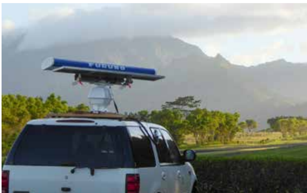
Figure 42. Radar unit mounted on a truck, being used to survey endangered seabirds on Kaua'i. Photo: Stephen Rossiter
