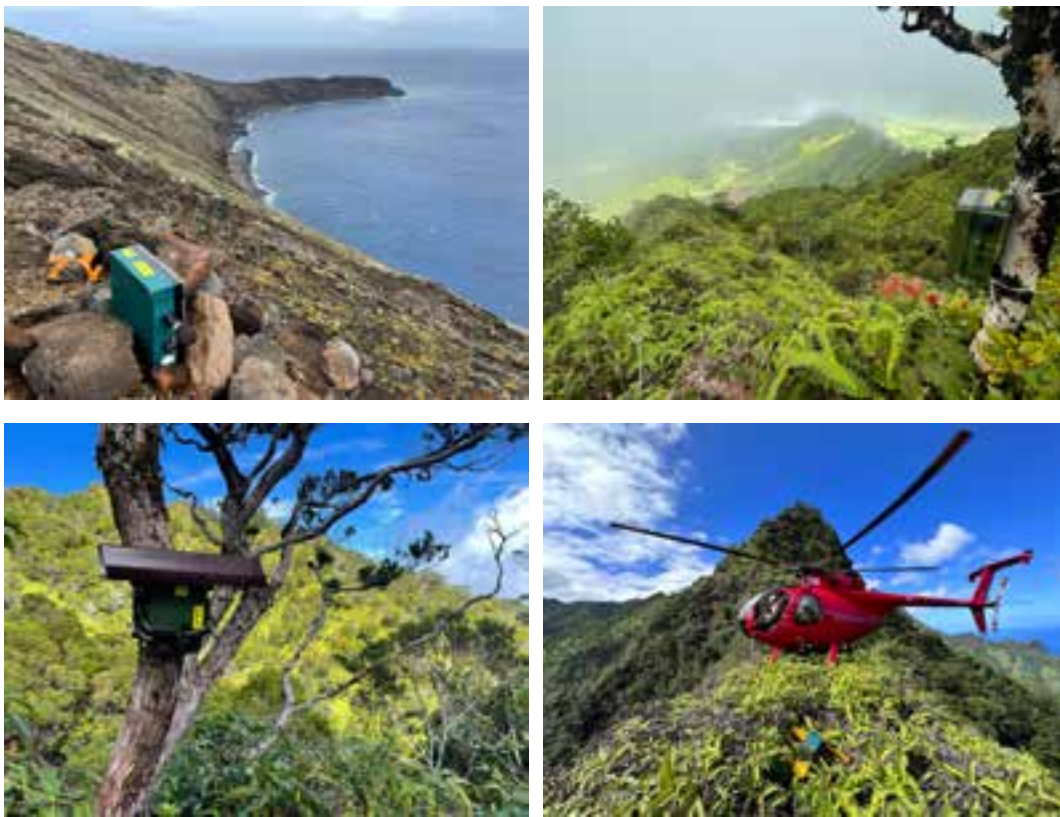
Figure 34. Examples of acoustic sensor deployments. Top left, on the ground on a dry poorly vegetated island. Top right, mounted on a tree in wet montane colony. Bottom left, on a tree in wet montane colony with dense understory. Bottom right, deployed from a helicopter in a specially designed deployment box. Photos: André Raine.
