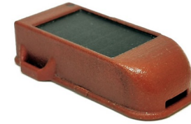
OrniTrack-20 - solar powered GPS-GSM (4G)
